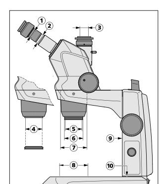
Fig. 4 Interfaces on the Stemi 508 with stand K (schematic diagram)
