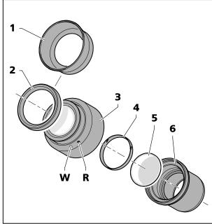
Inserting the eyepiece plate
