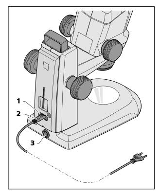
Fig. 12 Connecting the stereo microscope
