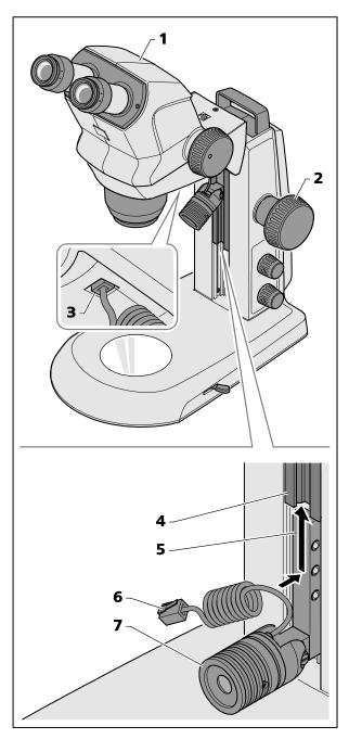
Fig. 8 Mounting spot illuminator
