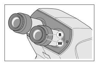
Fig. 14 Adjusting the eyepieces
