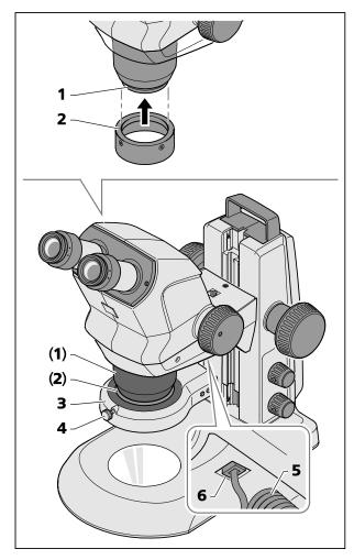
Fig. 9 Mounting ring illuminator
