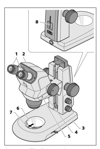
Fig. 6 Installing the stereo microscope
