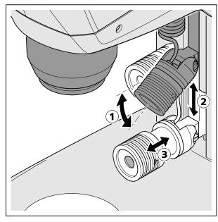
Fig. 15 Setting the spot illuminator
