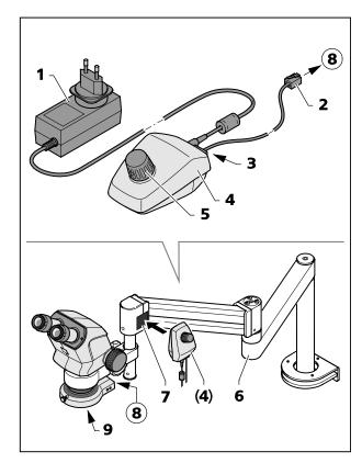
Fig. 18 Controller K LED
